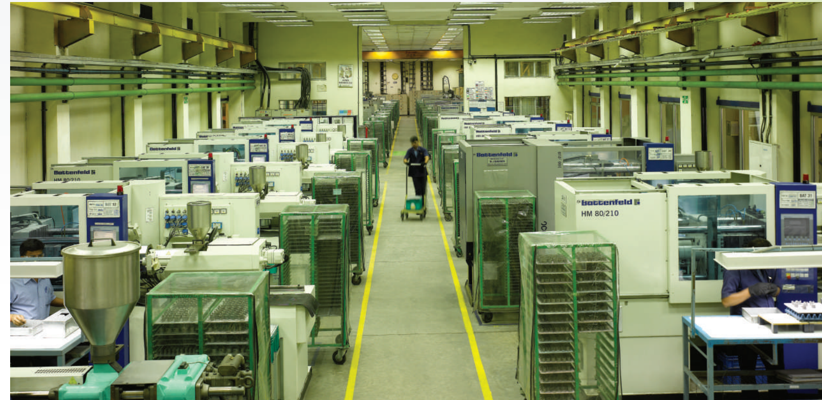
The injection molding bay of our Hoskote Operations contains the latest and most advanced closed loop injection molding machines available for MIM.
